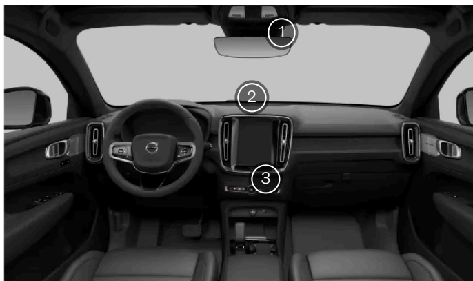
The interior climate sensors
