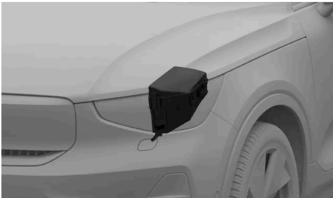
Fuse box location
