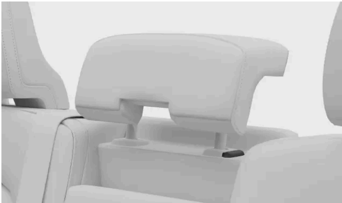
Locking button on the headrest
