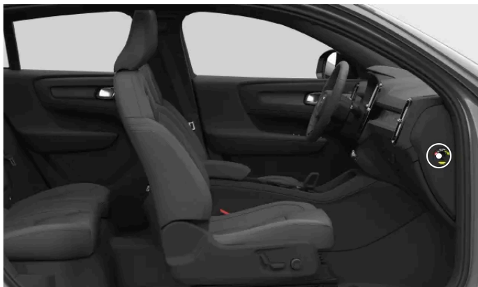
Location of the passenger airbag switch
