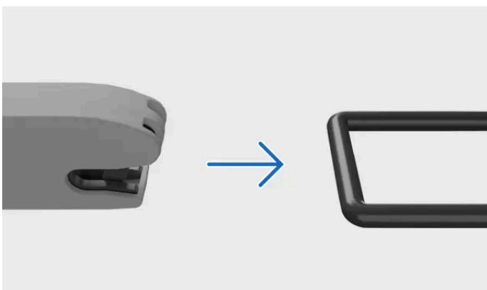
Attaching to ISOFIX anchorage point
