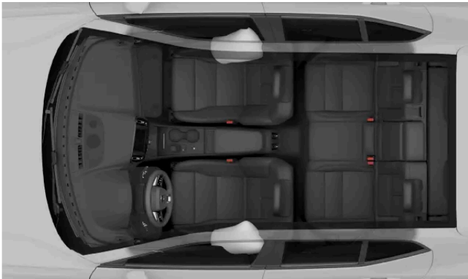
Side collision airbags for the front occupants.
