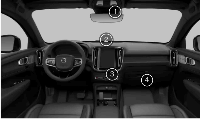
The interior climate sensors
