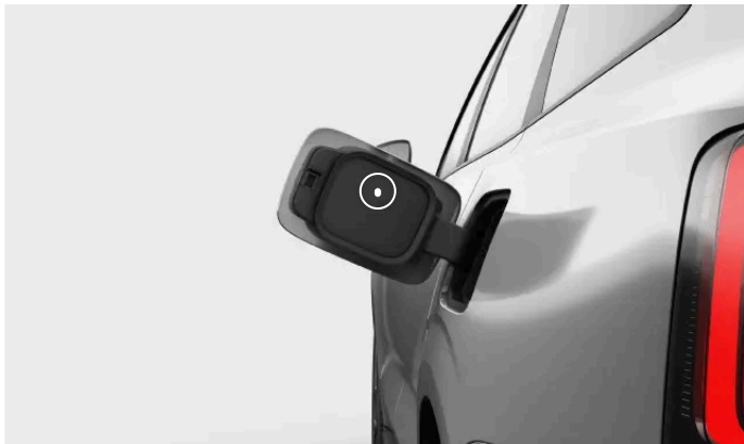
The identification label is located on the inside of the charging lid.
