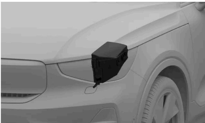
Fuse box location
