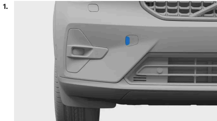
Front towing eye fastening cover
