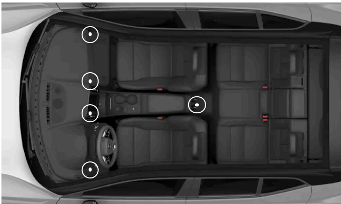
The locations of the adjustable air vents
