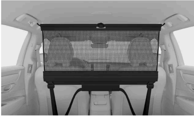
Installing behind second row seats
