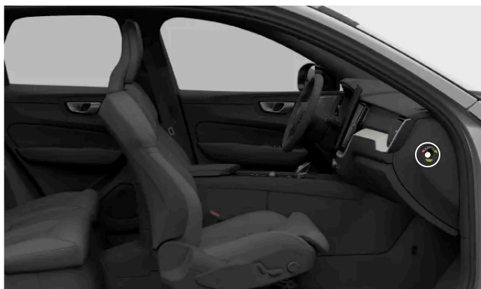
Location of the passenger airbag switch
