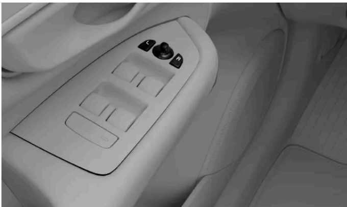
Controls for adjusting the wing mirrors
