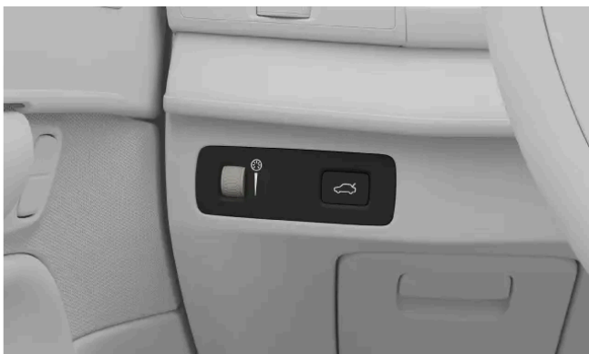
The interior lights adjustment thumbwheel
