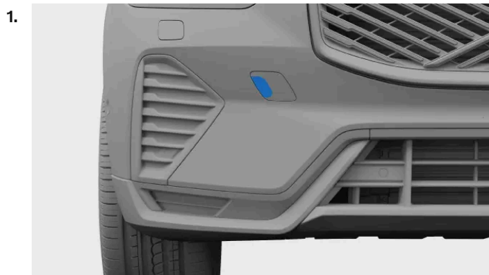
Front towing eye fastening cover
