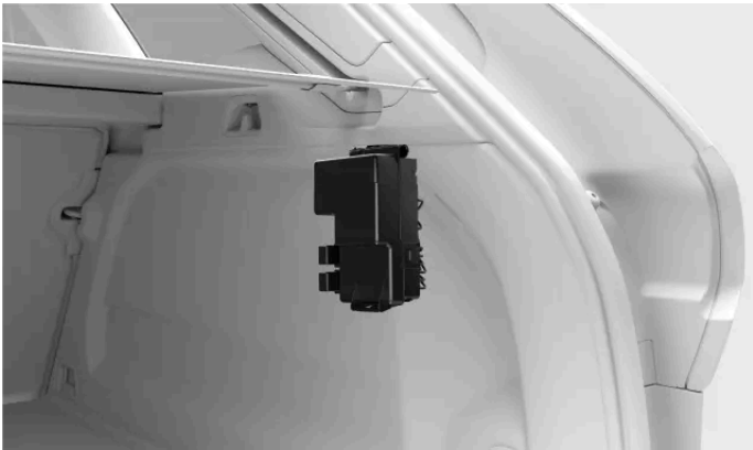
Fuse box location
