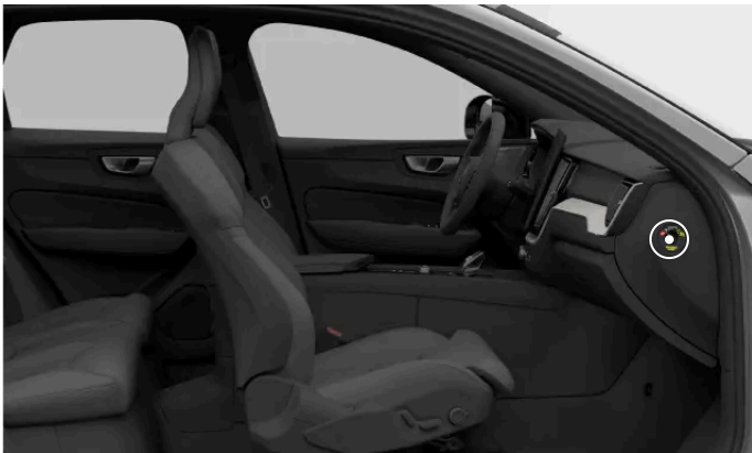
Location of the passenger airbag switch
