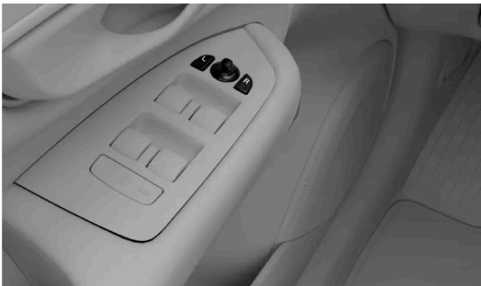
Controls for adjusting the wing mirrors
