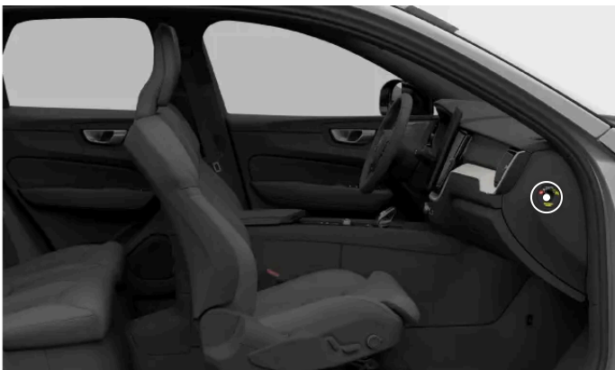
Location of the passenger airbag switch
