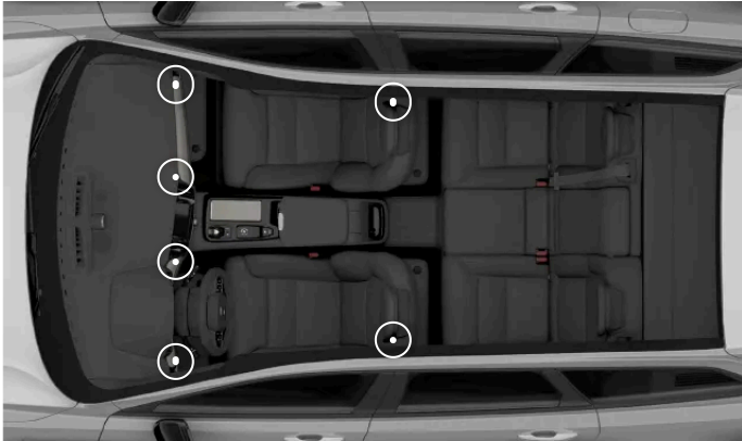
The locations of the adjustable air vents
