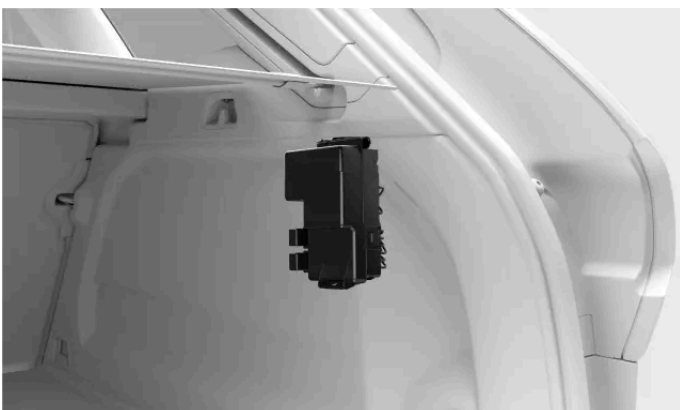
Fuse box location
