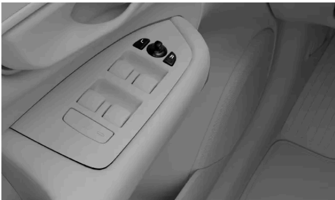
Controls for adjusting the wing mirrors
