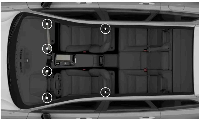
The locations of the adjustable air vents
