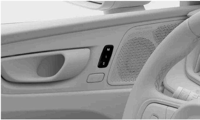
Location of the preset seat adjustment buttons
