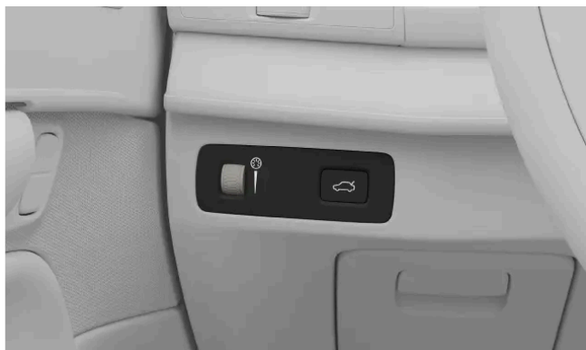
The interior lights adjustment thumbwheel
