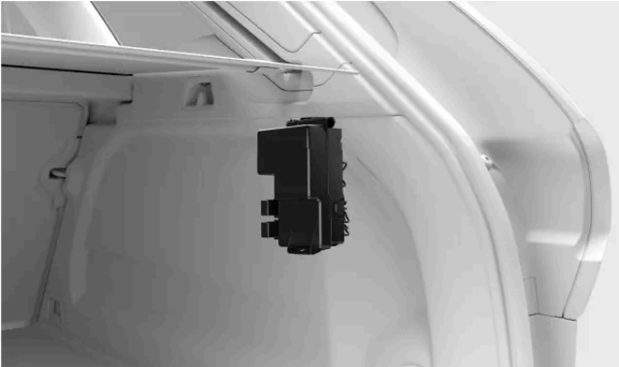
Fuse box location
