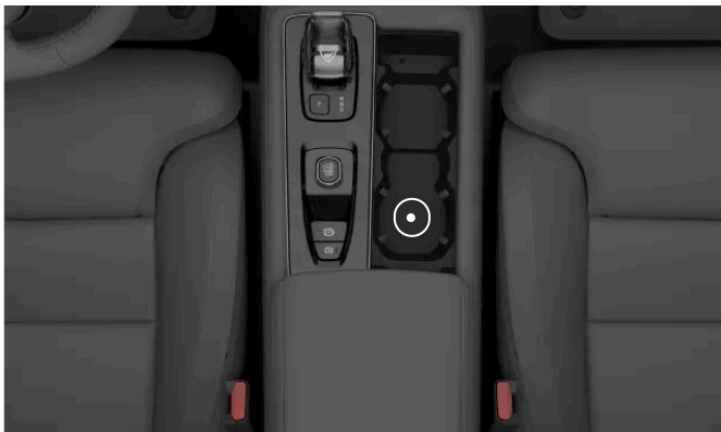
Location of the backup reader inside the tunnel console's cup holder
