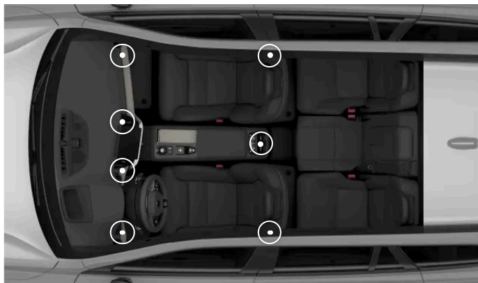
The locations of the adjustable air vents
