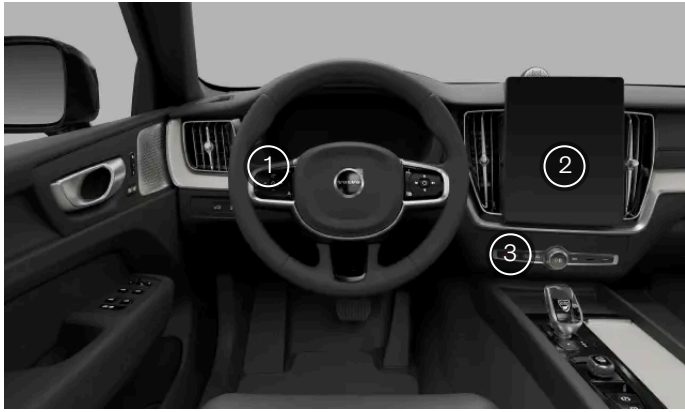
Exterior lights controls locations
