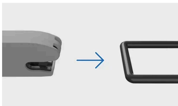
Attaching to ISOFIX anchorage point
