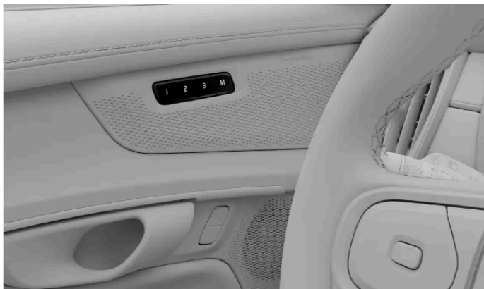
Location of the preset seat adjustment buttons
