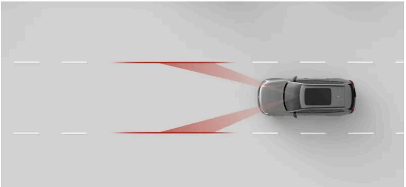
When lane keeping aid is enabled, the car can alert you if you are about to drift out of your lane and it can ask you to steer the car with attention. It can also perform steering interventions. Lane keeping aid relies on the car's forward-facing camera to identify road markings and your position in the lane.
