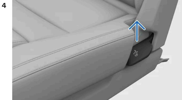
Pull and hold the handle on the side of the seat upwards to unlock backrest movement.
