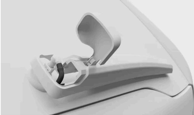
Find the plastic cover where the wiper arm attaches to the car. Loosen the side of the cover closest to you first and then the side furthest away from you. Lift the plastic cover up fully. This will give you access to the hose connector.
