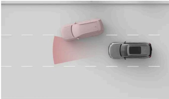
The front radar's detection zone has a limited width. If you get cut off by another vehicle, detection can occur relatively late causing a sudden response by your car.
