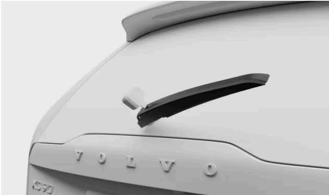
Grasp the centre of the wiper arm and lift it up and away from the rear windscreen. You may feel some resistance halfway – this is the lock position. You need to pull the wiper arm past the lock position so that it doesn't fall back onto the windscreen.
