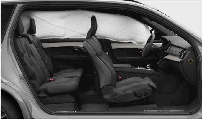
Inflatable curtain deployed on one side of the car.
