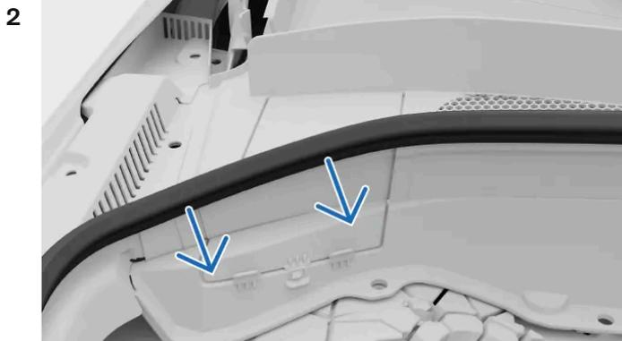
The coolant container is located in the upper-left corner of the engine compartment, underneath a panel hatch. Pull the rubber seal towards the engine compartment to access the hatch.
