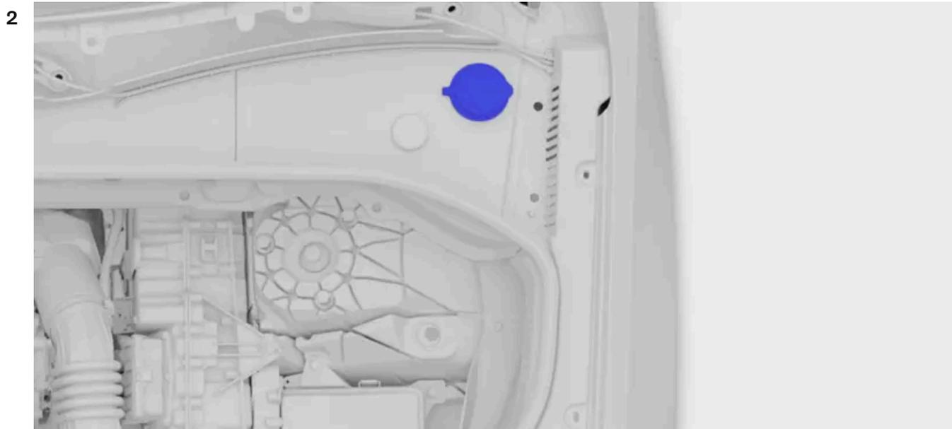
Locate the blue cap with the washer fluid symbol and open it.
