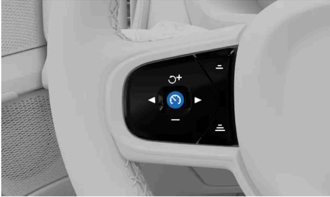
When it's safe to do so, press the Pilot Assist button
