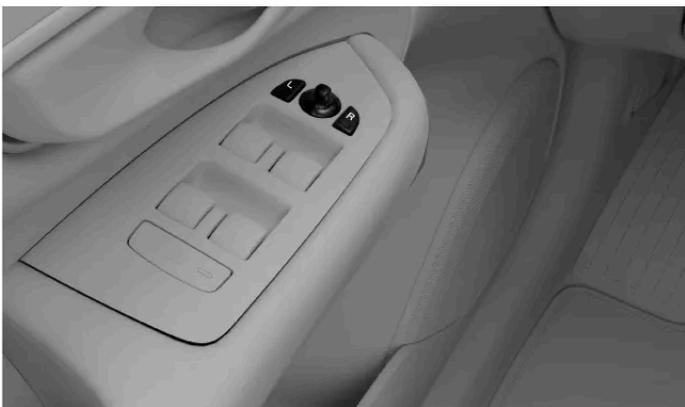
Controls for adjusting the wing mirrors
