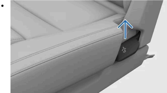
Pull the handle on the side of the seat upwards.
