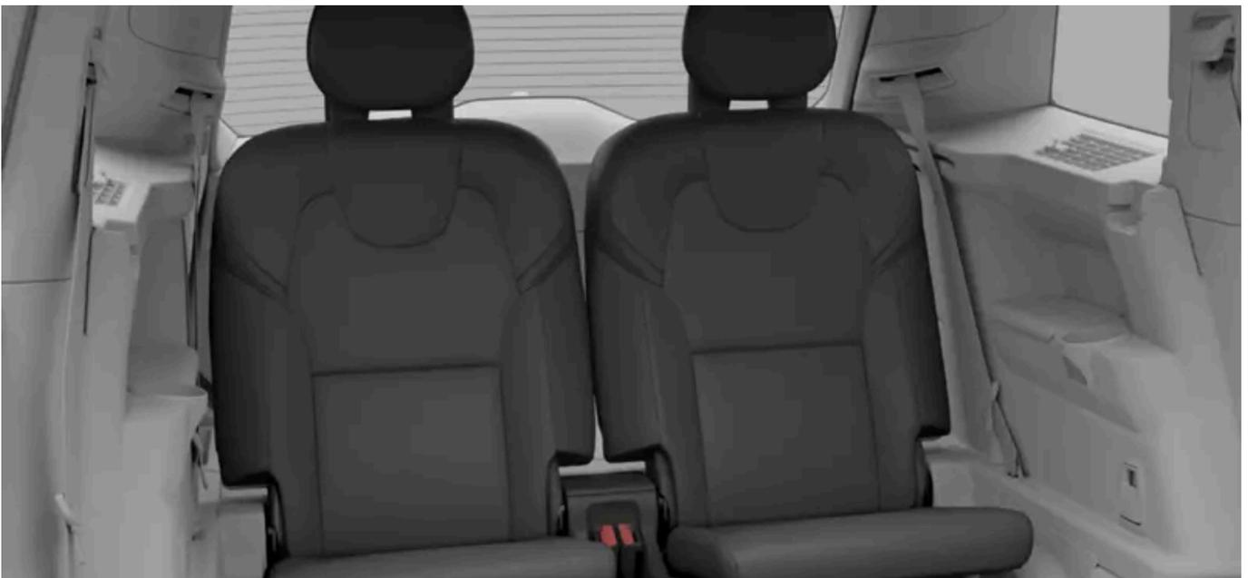
The backrests and headrests can fold in one motion to give you more stowing space. The headrest folds down automatically when the backrest is lowered.
