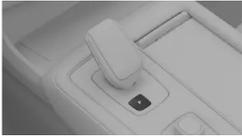
When P is selected, the gearbox is mechanically blocked to avoid accidental gear shifts.
