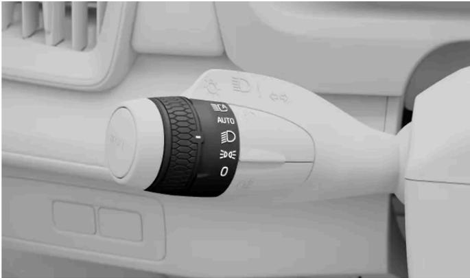
The passing beam symbol on the rotating ring on the left-hand stalk
