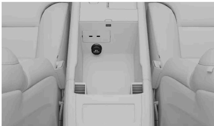
The 12 V electrical socket in the tunnel console
