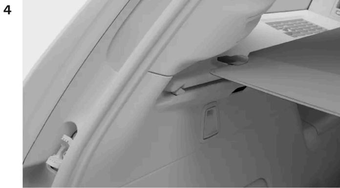
Slide the ends of the load cover screen into the upper grooves of the side panels.
