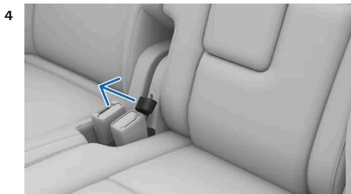
Pull and hold the strap on the side of the seat to unlock backrest movement.
