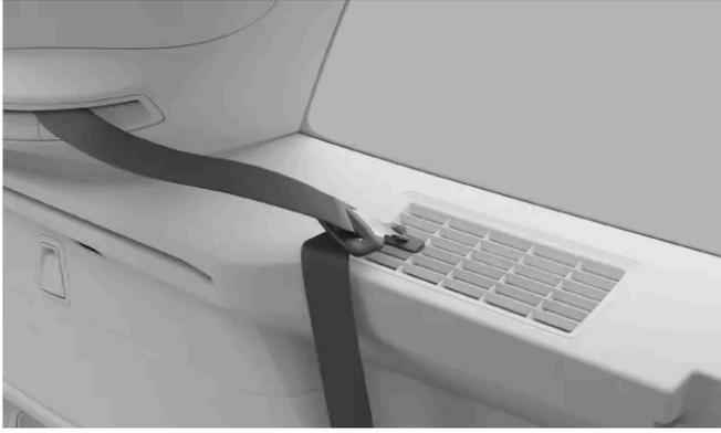
Keep the third row seatbelt out of the way when using the load cover. Pull the seatbelt back and hang it on the belt knob.
