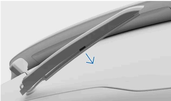
Pull the blade down until it loosens and comes away from the wiper arm.
