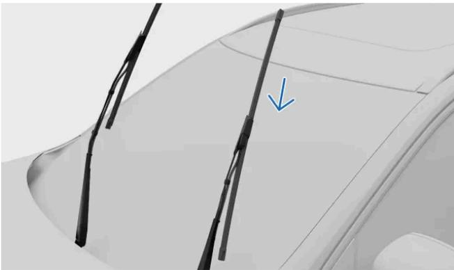
Make sure that the blade for the driver side is longer than the blade for the passenger side. Slide the wiper blade onto the wiper arm. Ensure that the pin on the wiper arm goes into the hole on the wiper blade. Push the blade into the wiper arm until you hear a click sound.
