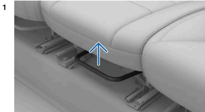
Grasp and pull the handle under the seat cushion upwards.
