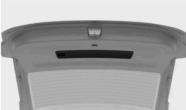
The warning triangle is located on the inside of the boot hatch. Open the compartment by turning the handle so that it's vertical and then pulling it.
