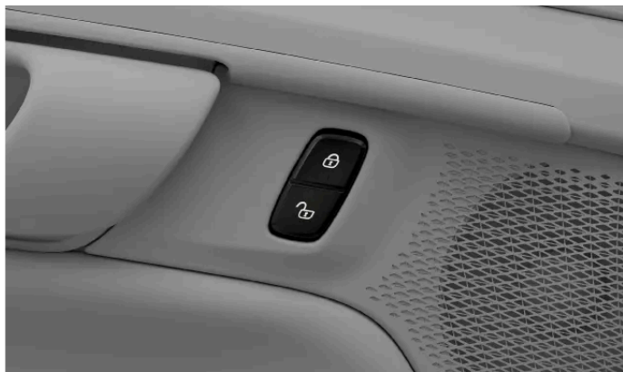
Front door button for central locking
