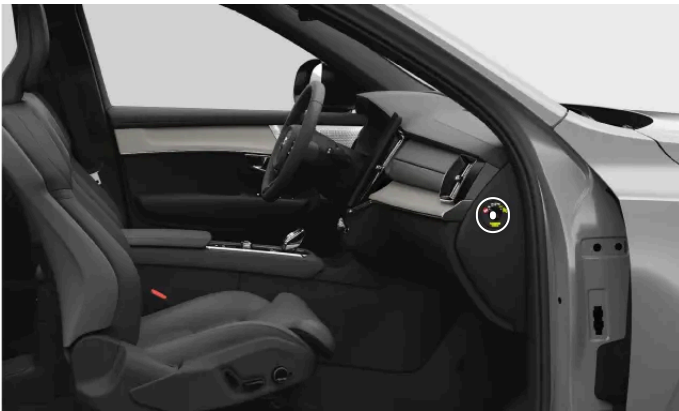
Location of the passenger airbag switch
