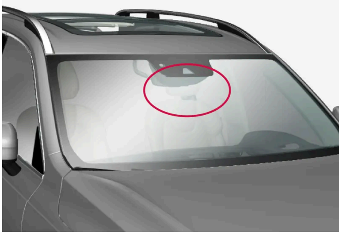
Location of the camera unit
