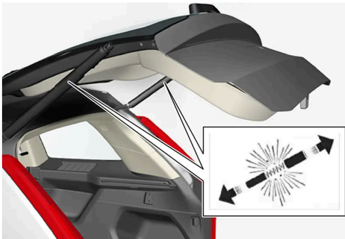
The pre-tensioned springs for the power operated tailgate.
