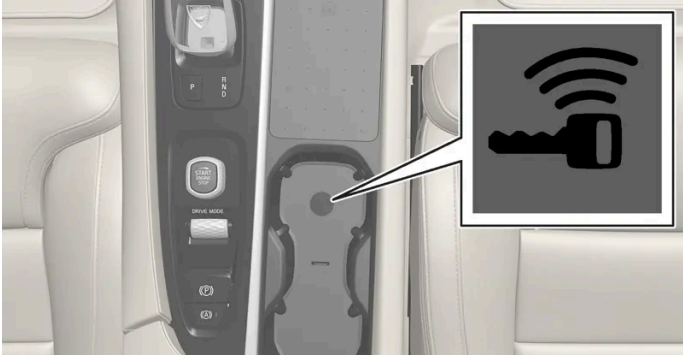
Backup reader's location in the tunnel console.
