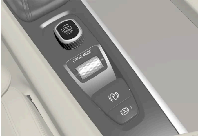
Start knob in the tunnel console.
