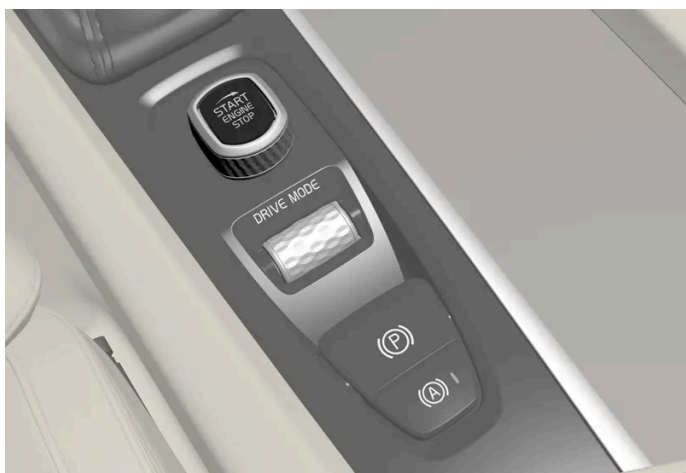
Start knob in the tunnel console.
