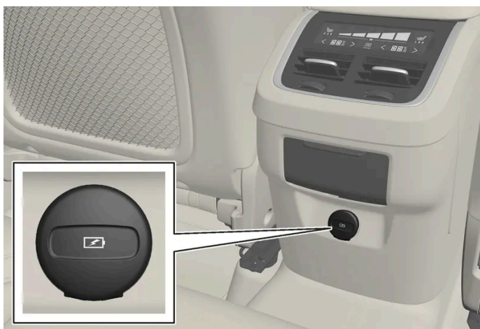
USB ports (type C) on rear of tunnel console for charging phones and tablets [1] , for example.
