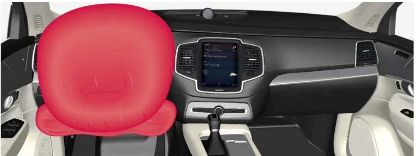
Steering wheel airbag and knee airbag on the driver's side in the front seat.
