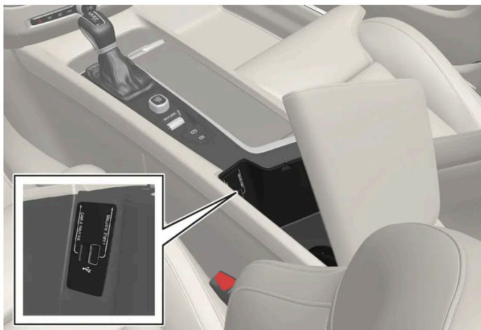
USB ports (type A) in the tunnel console. Allow the cable to lie forwards so that it is not trapped when the lid is closed.
