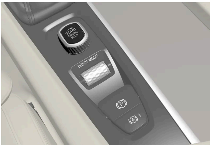
Start knob in the tunnel console.
