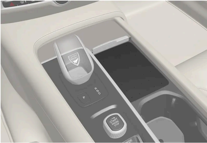
Wireless phone charger in the tunnel console.
