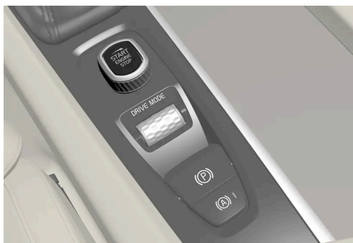
Start knob in the tunnel console.
