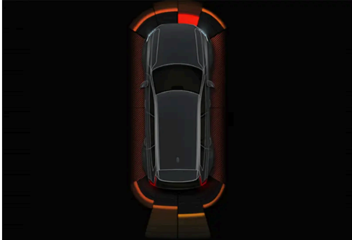
Example of screen view with obstacle zones and sensor sectors.
