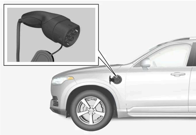
Charging cable handle and charging input socket.
