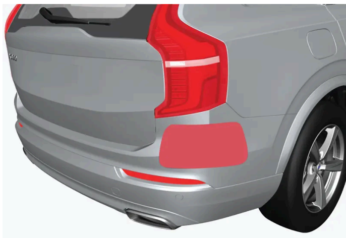
Location of rear radar units
