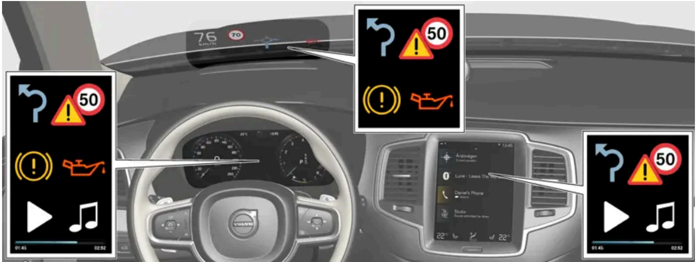
Different types of information are shown in different displays depending on how the information should be prioritised.
