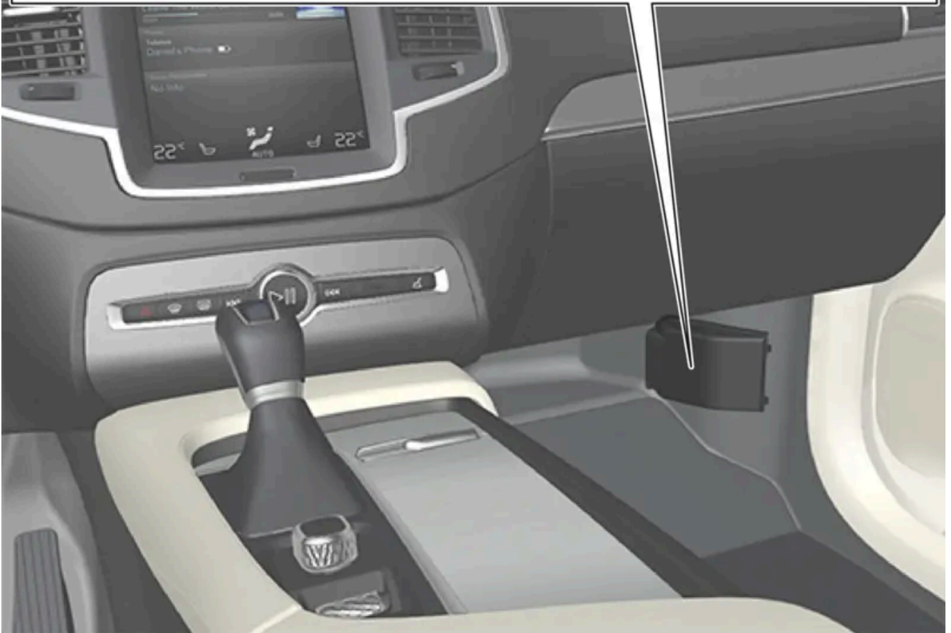
The central electrical unit is located behind the floor mat/side panel.
