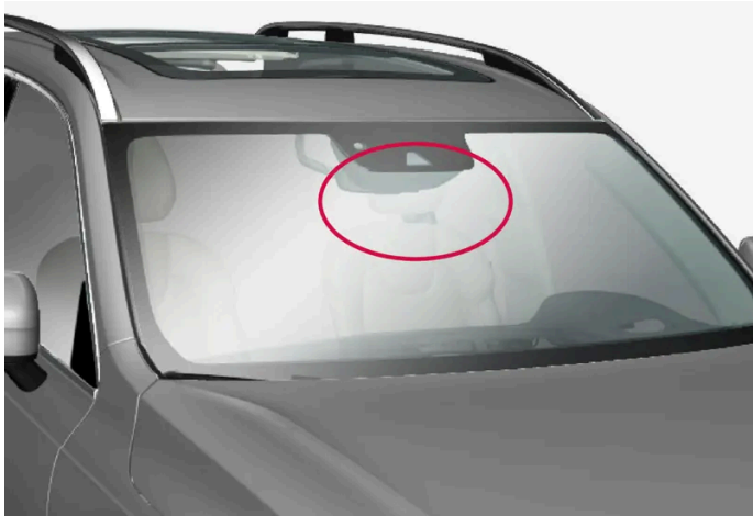
Location of front radar unit
