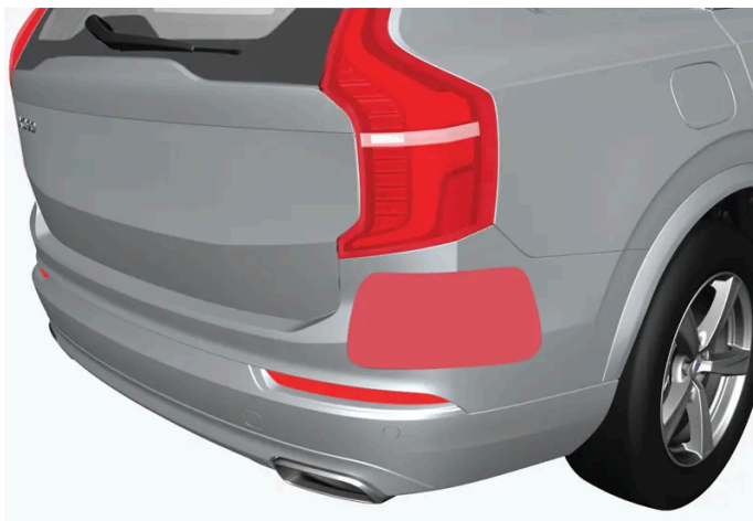
Location of rear radar units
