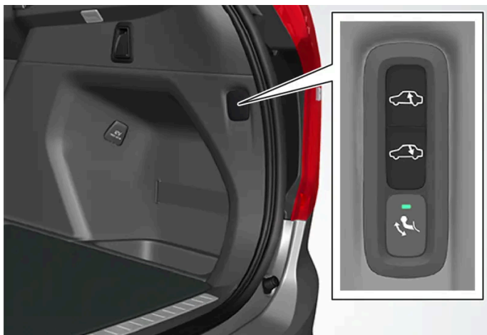
Controls for raising/lowering the car's rear section.
