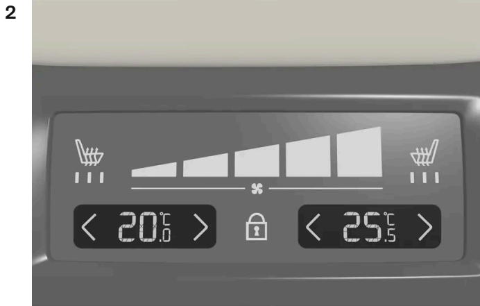
Temperature control on the climate panel at the rear of the tunnel console.
