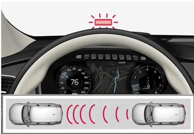
Warning light for distance warning is shown on the windscreen.
