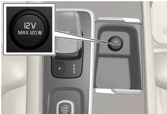
The tunnel console's front electrical socket for cars without wireless phone charger*.
