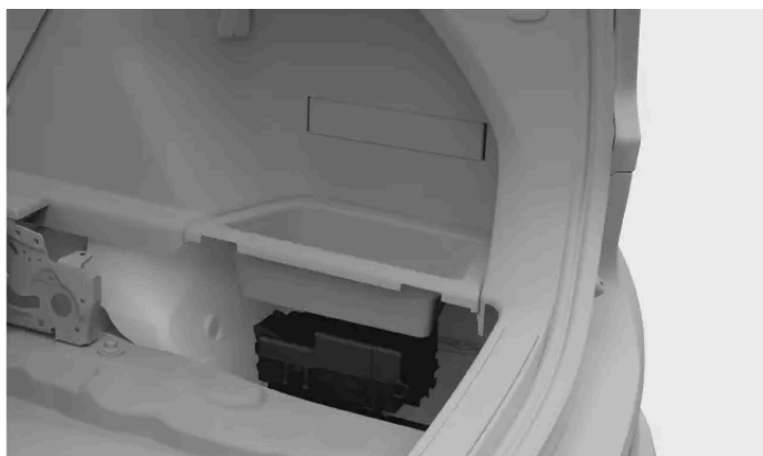
Fuse box location
