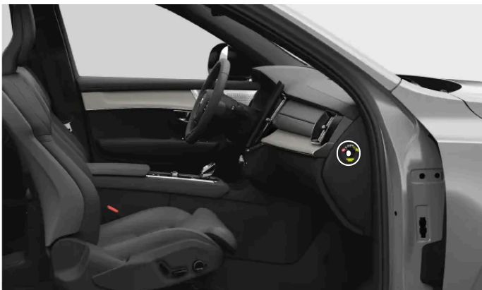
Location of the passenger airbag switch
