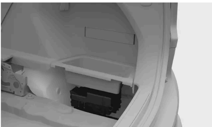
Fuse box location
