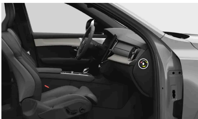
Location of the passenger airbag switch
