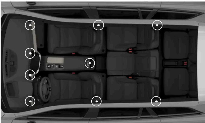
The locations of the adjustable air vents
