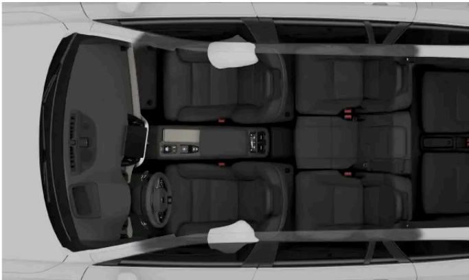
Side collision airbags for the front occupants.
