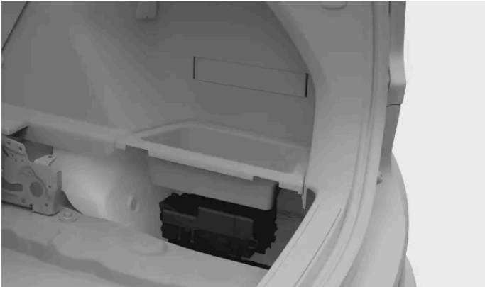
Fuse box location
