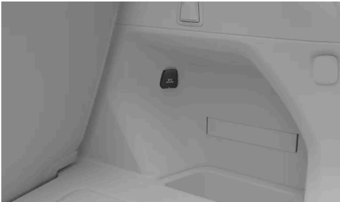
The 12 V electrical socket on the right-hand side in the boot
