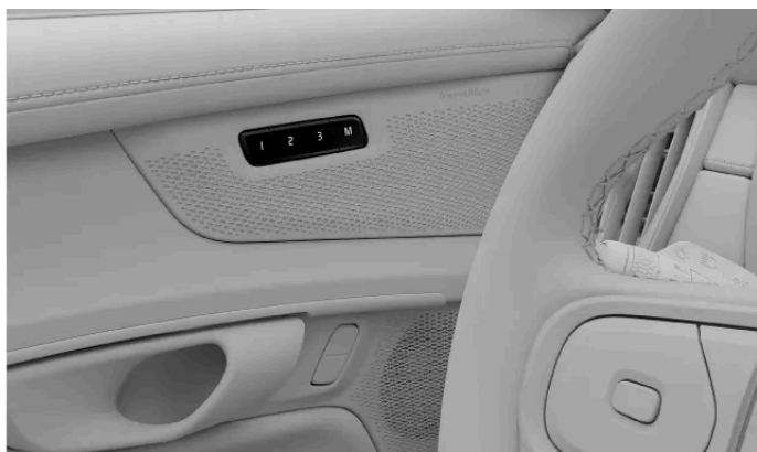
Location of the preset seat adjustment buttons
