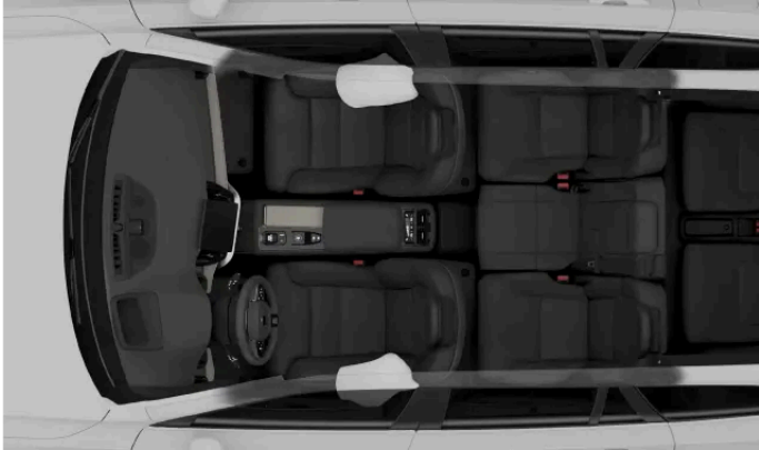
Side collision airbags for the front occupants.
