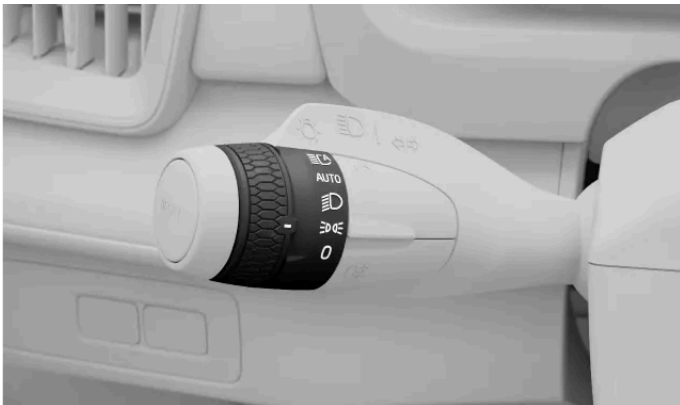
The position lights symbol on the rotating ring on the left-hand stalk
