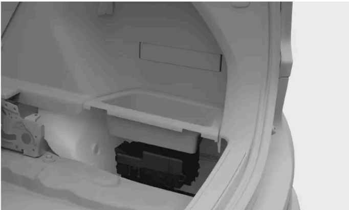
Fuse box location
