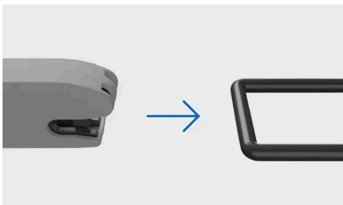
Attaching to ISOFIX anchorage point
