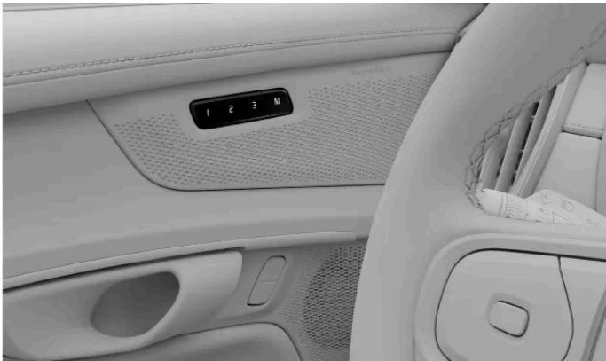
Location of the preset seat adjustment buttons
