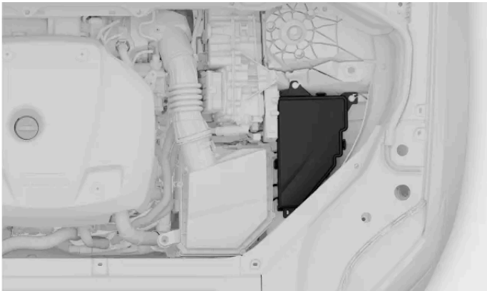
Fuse box location
