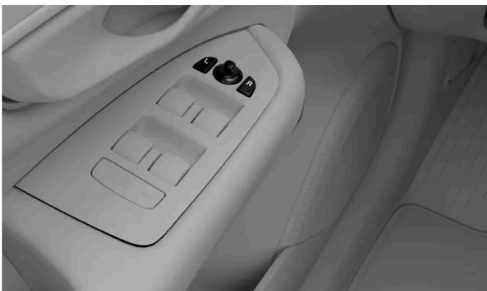
Controls for adjusting the wing mirrors
