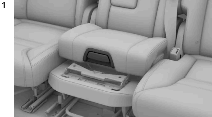
Pull the handle on the front of the child seat to release the lock.
