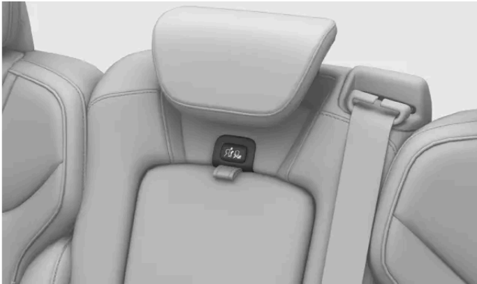
Locking button on the centre headrest
