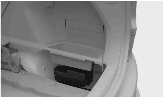
Fuse box location
