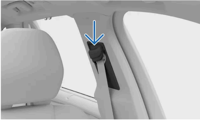
Seatbelt upper anchor point
