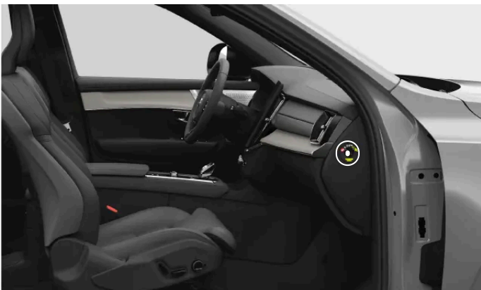
Location of the passenger airbag switch
