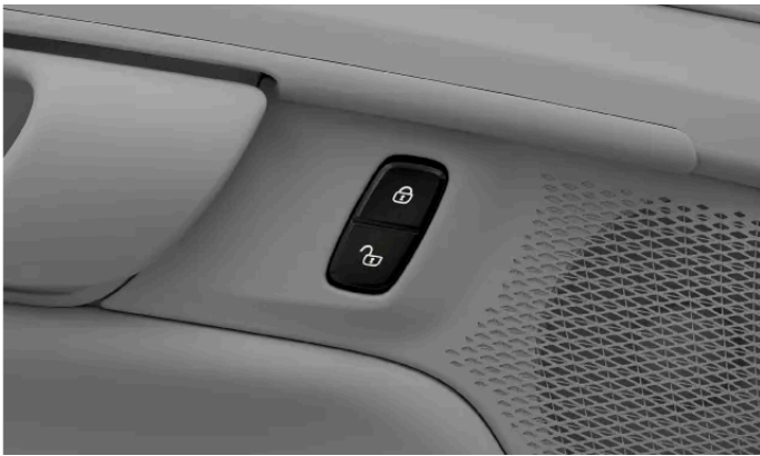
Front door button for central locking
