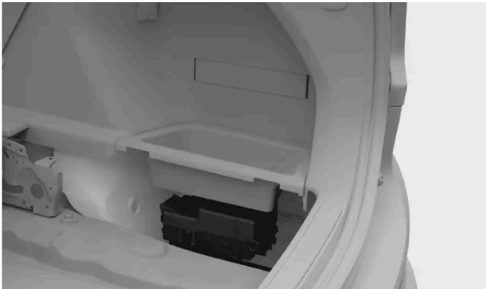
Fuse box location
