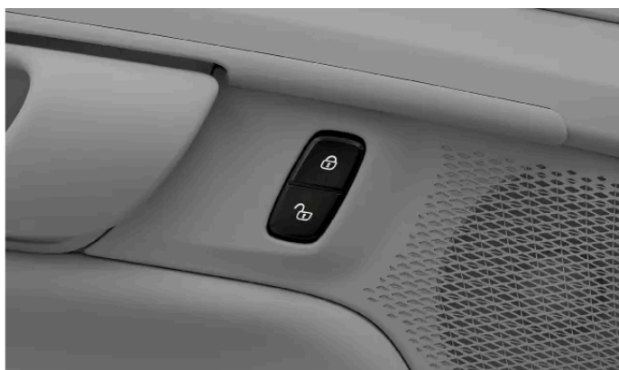
Front door button for central locking
