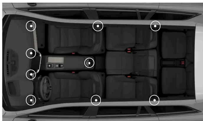
The locations of the adjustable air vents
