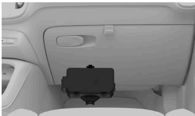
Fuse box location
