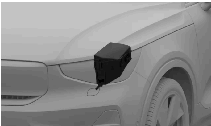
Fuse box location
