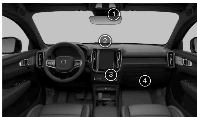
Interior climate sensors
