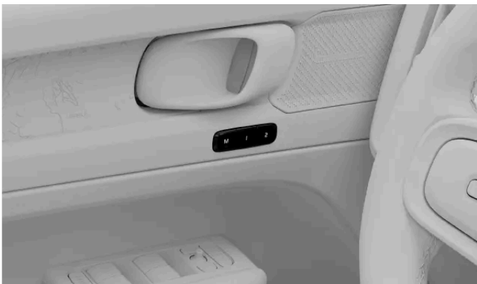
Location of the preset seat adjustment buttons
