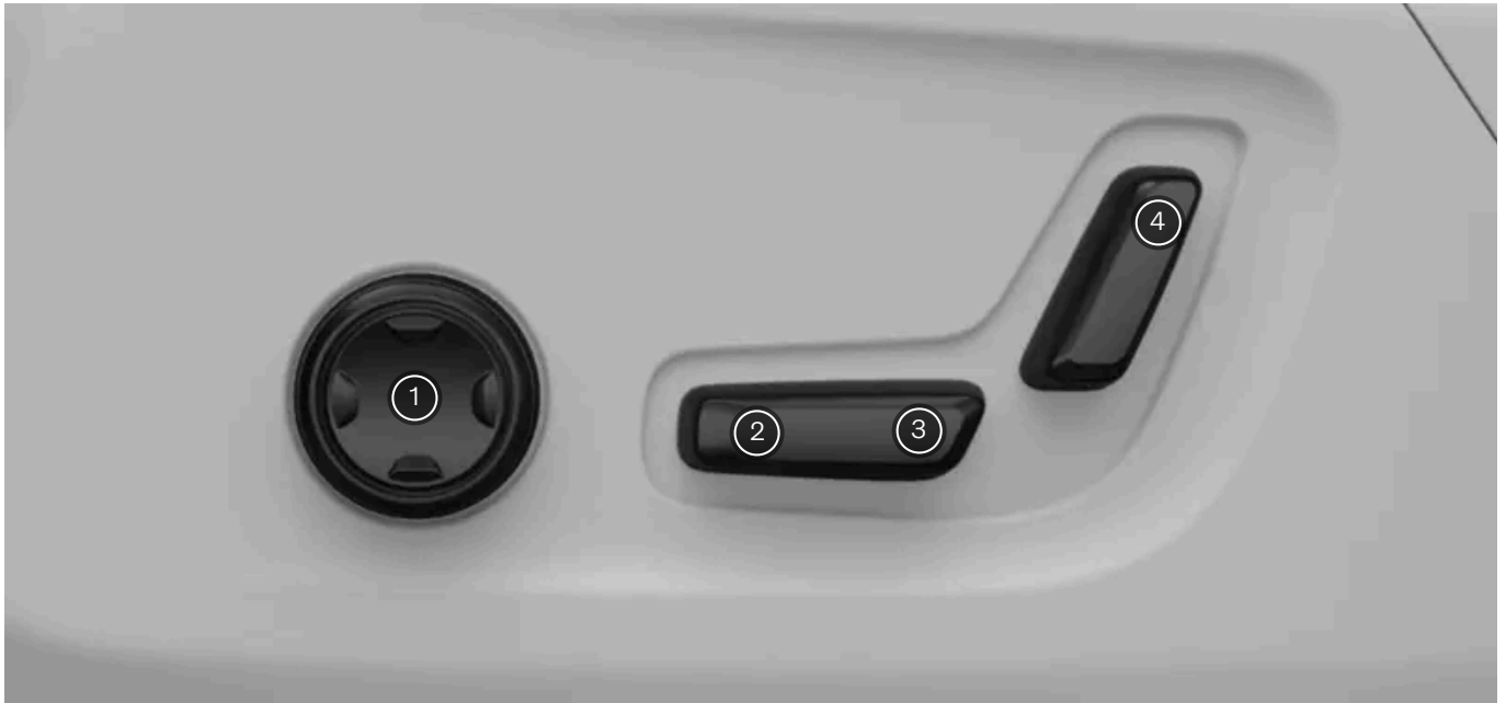
Controls on the side of the seat
