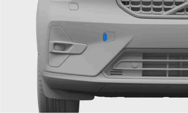
Front towing eye fastening cover
