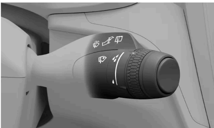
Right-hand steering wheel stalk
