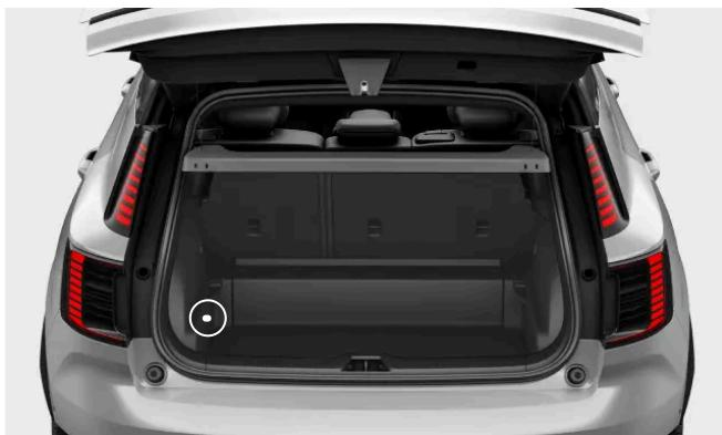
**3** Remove the cap by prying it off with a screwdriver or a similar tool.
