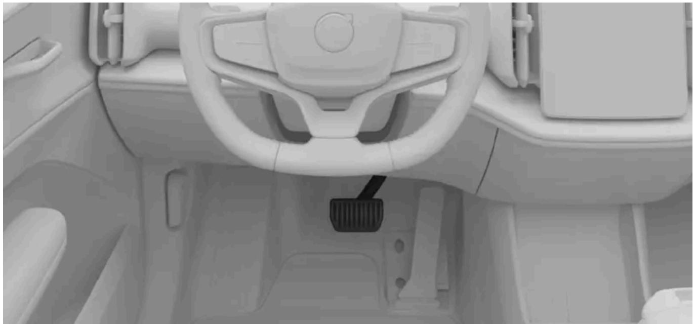
The foot brake engages either regenerative braking or the friction brakes, depending on how hard you press the pedal. Light braking activates regenerative braking, whereas harder braking engages the friction brakes.
