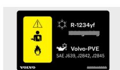
The label with information on climate system fluids is located under the hood, on the right-hand side of the vehicle.
