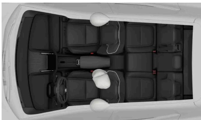
Side-on collision airbags for the front occupants.
