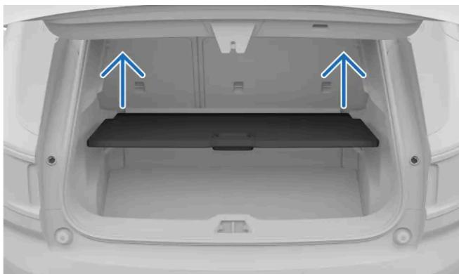
Illustrated guide to removing the cargo hatch.
