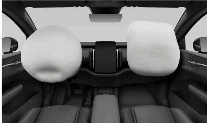
The driver side airbag is packed inside the steering wheel.
