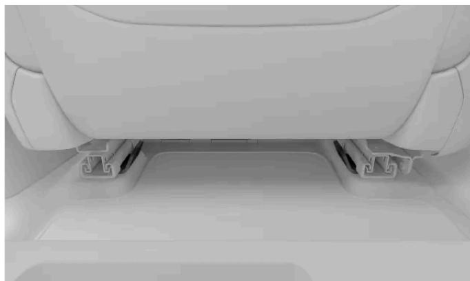
The lower tether attachment points for the rear seats can be found at the back of the floor rails of the seats in front.
