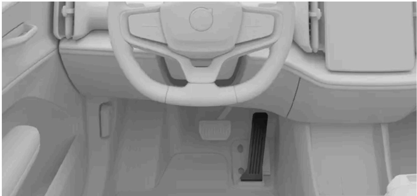
Braking behavior changes through the use of the accelerator pedal. When you press the accelerator, the vehicle accelerates normally, but releasing the pedal engages braking. The more you ease up on the pedal, the more braking action you get.
