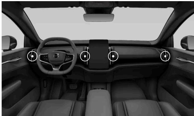
The positions of the adjustable air vents.
