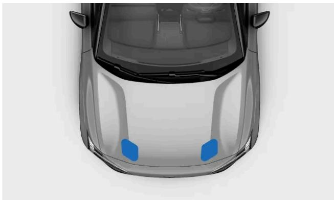
Press down with both hands on the front edge of the hood. Make sure the hood fits into the latches at the same time. Keep the front edge flat as it closes.
