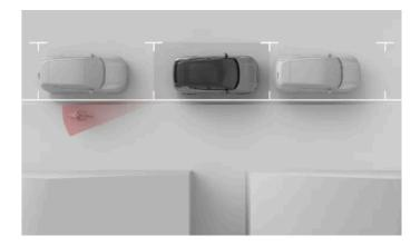
Door opening alerts are designed to warn you of passing traffic so that you don't open a door in its path. These alerts can be provided when the vehicle is stationary or moving very slowly [1].
