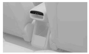
From the rear seats, you can operate the rear windows using the switches at the back of the center armrest.
