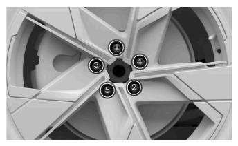
Tighten the wheel fasteners crosswise.
