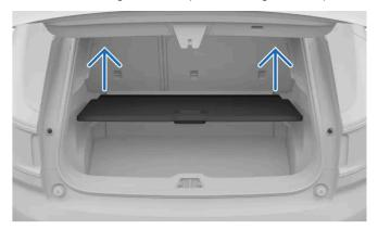
Illustrated guide to removing the cargo hatch.
