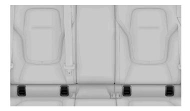
The ISOFIX<sup>[1]</sup> attachment points for the rear seats are located behind a flap in the lower part of the backrest on the outer rear seats. The flap needs to be unfolded to access the anchor points behind it.
