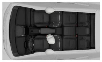
Side-on collision airbags for the front occupants.
