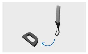
Fastening tether to lower tether attachment point
