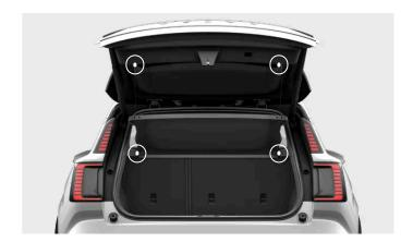
There are two attachment points on the parcel shelf itself and two on the trunk hatch. When the parcel shelf is attached, cords run between attachment points on the parcel shelf and the trunk hatch.
