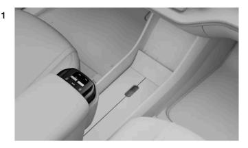
From the front seats, you can control all of the power windows. Press the button with the text REAR to switch between operating the front or rear windows. The button turns amber to indicate that the rear windows are selected. The controls will switch back to the front windows if you press the button again or after a few seconds of inactivity.
