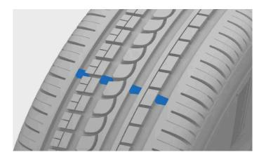
The narrow grooves that run lengthwise across the tire's tread pattern are tread wear indicators. On the side of the tire are the letters TWI<sup>[1]</sup>.
