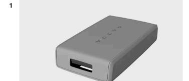
Hold the tag with the Volvo logo facing upwards. There is a small opening on one of the tag's short sides. Pry open the tag from this side by pulling the edge outwards and upwards.
