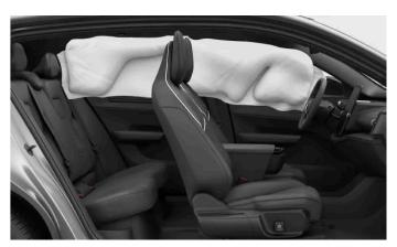
Inflatable curtain deployed on one side of the vehicle.
