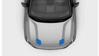
Press down with both hands on the front edge of the hood. Make sure the hood fits into the latches at the same time. Keep the front edge flat as it closes.
