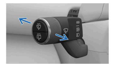
You can move the left-hand stalk forward or backward to switch between the different high beam options. The stalk always springs back to the neutral position.
