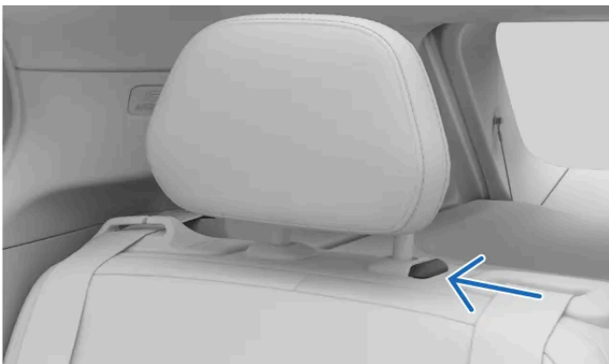
Locking button on the headrest
